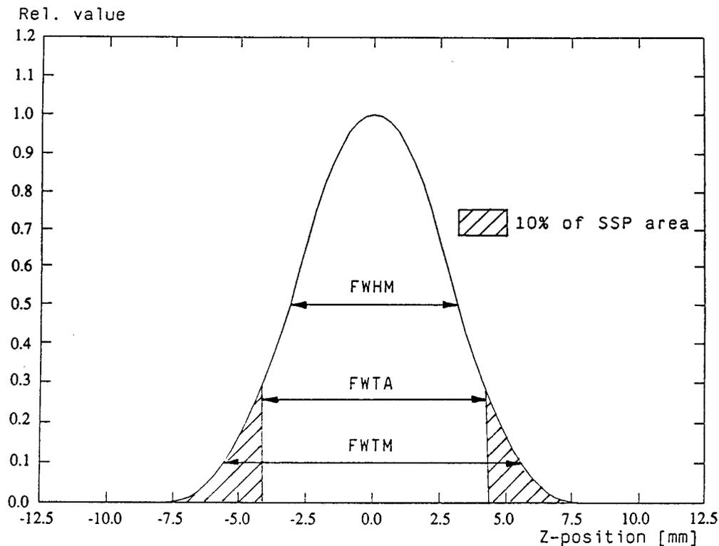
FIG. 1. Width descriptors of the section sensitivity profile (SSP). The full width at half-maximum (FWHM) typically is used to describe the nominal scan width. The FWTM is the full width at one-tenth of the maximum, and the FWTA is defined as the width between points on the profiles which include 90% of the area and exclude 10% of the area under the entire profile. [From Polacin *et al.* (Ref. 7). By permission of Radiological Society of North America.]
