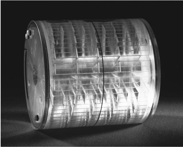
FIG. 2. The section thickness and contiguity phantom (Ref. 9) used to visually demonstrate changes in the section sensitivity profiles.
